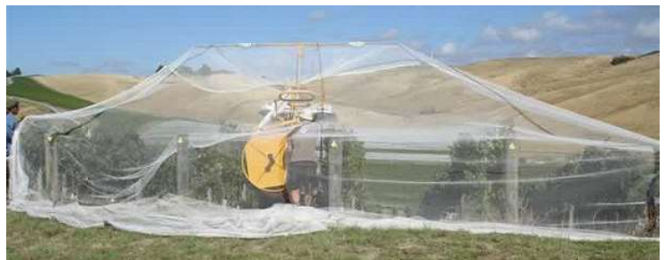
Netwizz Slim Auto Tension, covering five rows (old model pictured)
