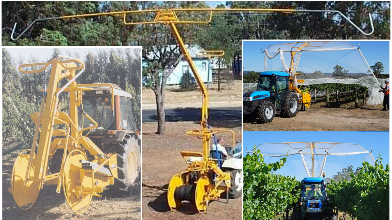
High Lift top arms fold back, mast retracted then lowered.
