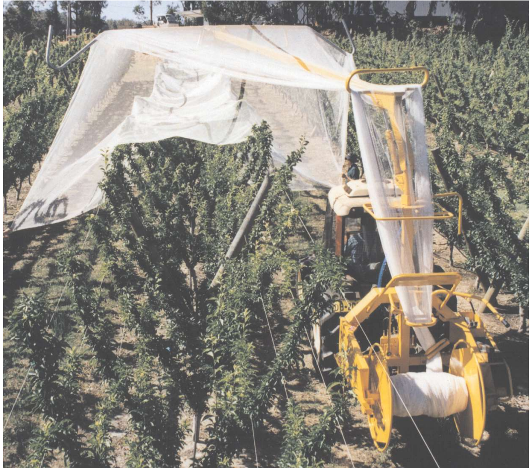
covering single row Tatura trellis, with mast offset 30°
