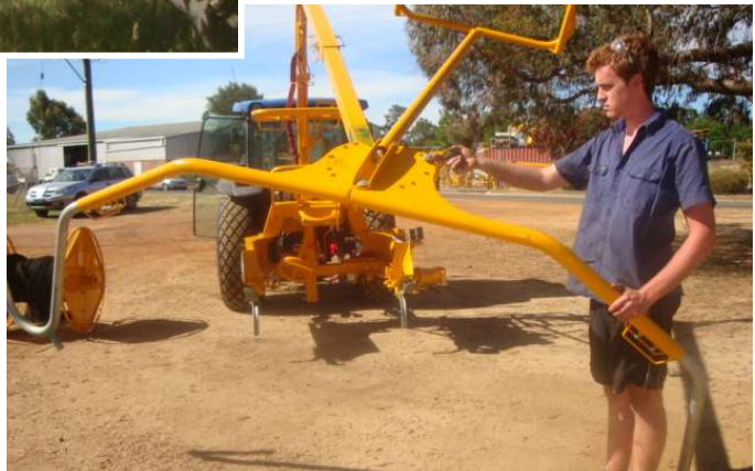
Rotating the top head assembly can be set at 0°, 30° or 45°
