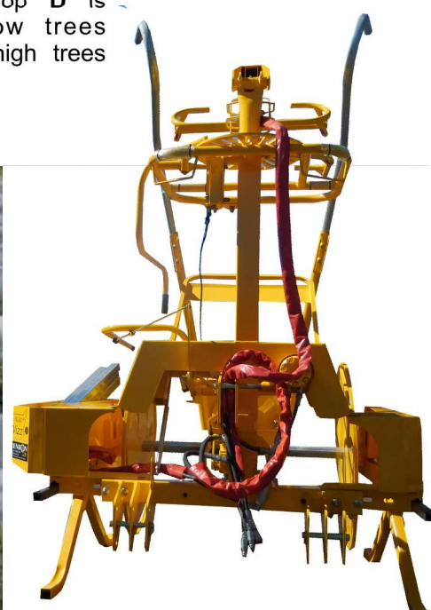
NetWizz High Lift Swivel Head folded up in the 1.4m spindle length setting (1.85m outside) as pictured above
